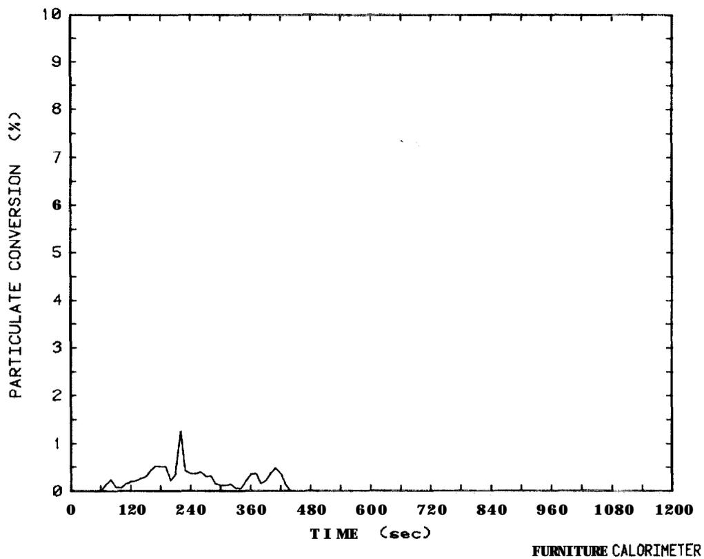
Figure 102. Smoke particulate conversion plot for 12.7 mm plywood wardrobe, Test 43
