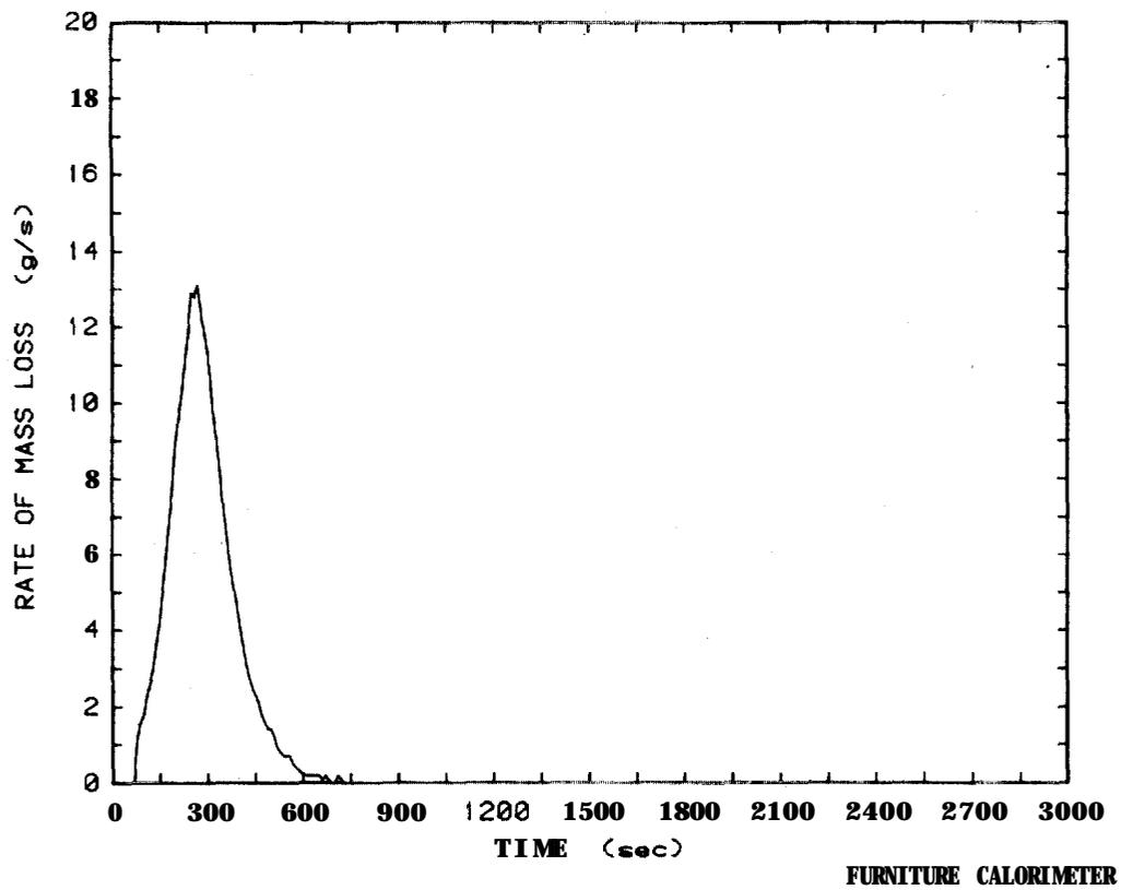
Figure 45: Rate of mass loss plot for metal frame chair, Test 53
