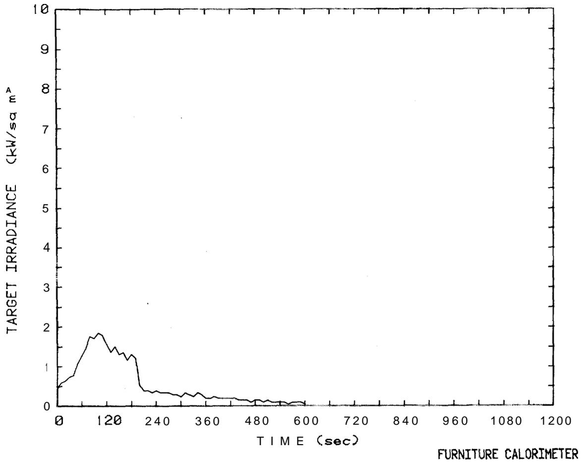
Figure 37. Target irradiance plot for molded fiberglass chair
