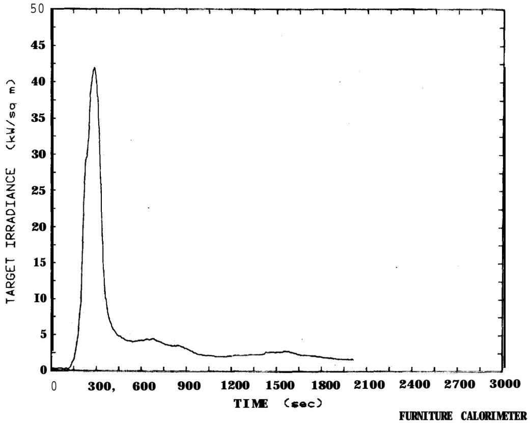
Figure 5: Target irradiance plot for easy chair, Test 45
