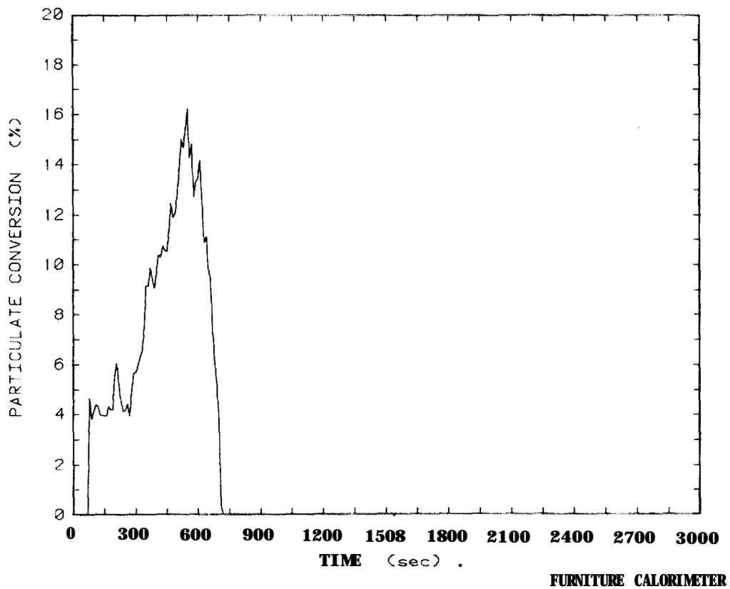
Figure 11: Smoke particulate conversion plot for Test 48
