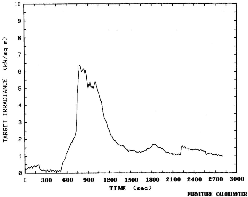
Figure 76. Target irradiance plot for wood frame loveseat, Test 57
