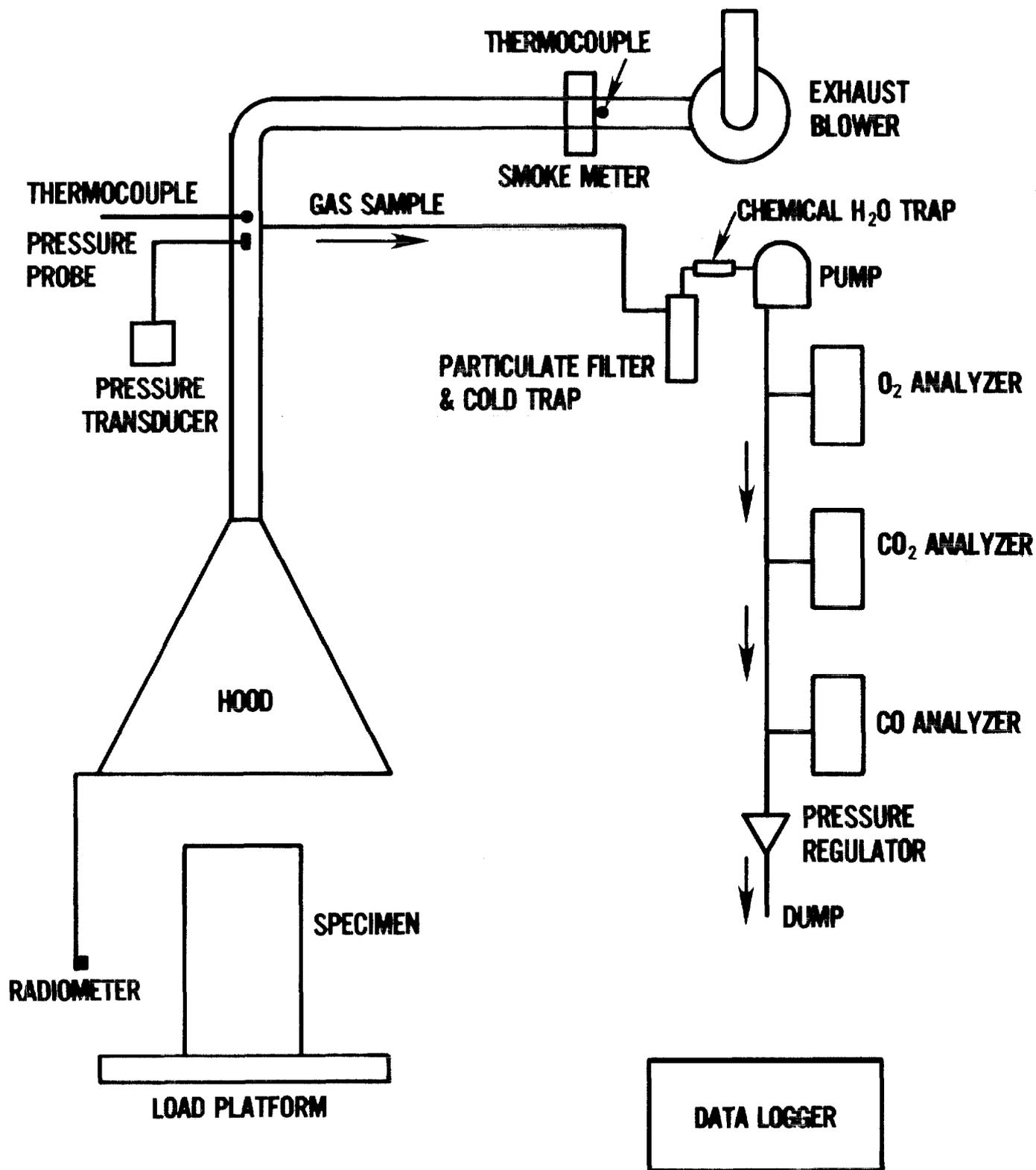
Figure 1. Furniture calorimeter, schematic of flow and instrumentation
