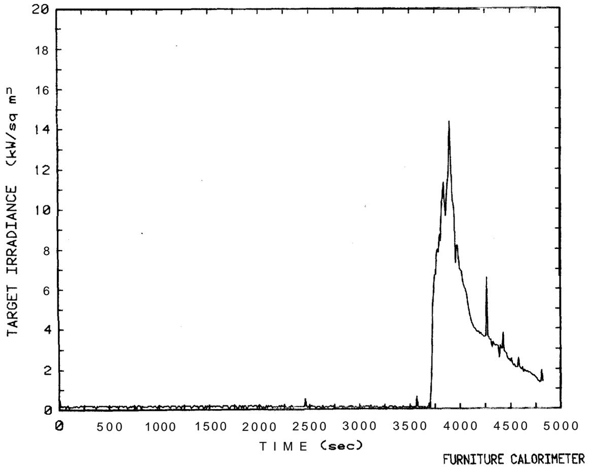
Figure 25. Target irradiance plot for easy chair Test 66
