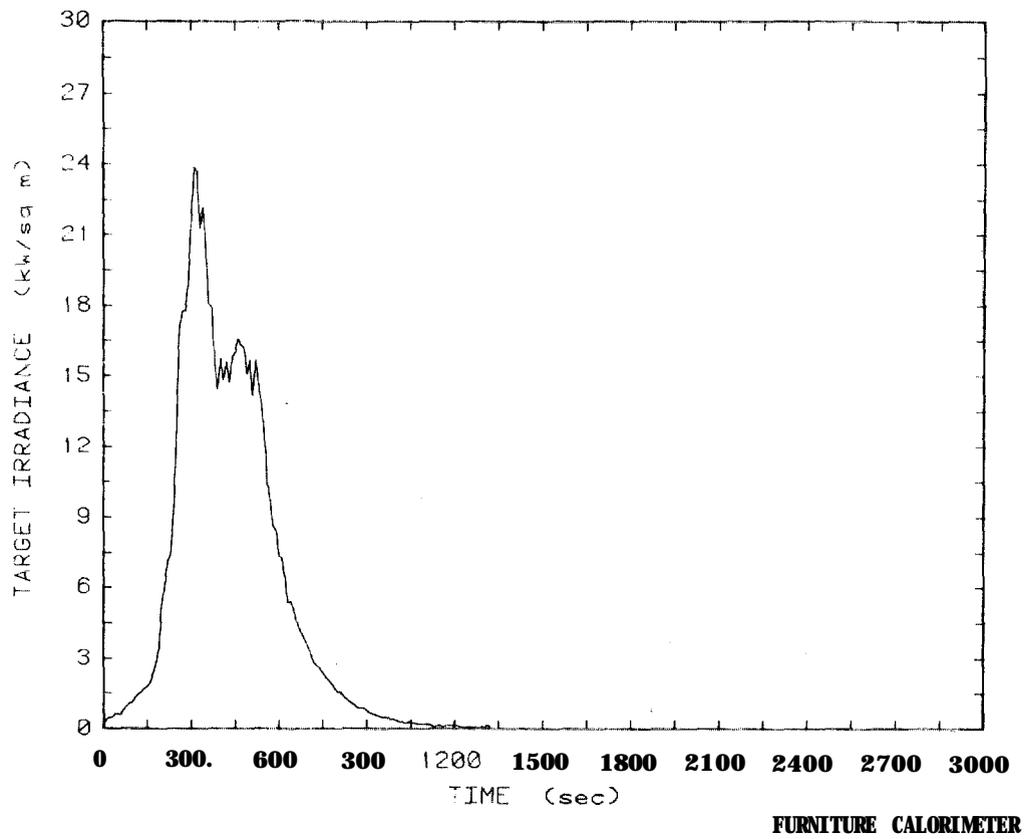
Figure 10: Target irradiance plot for easy chair, Test 48
