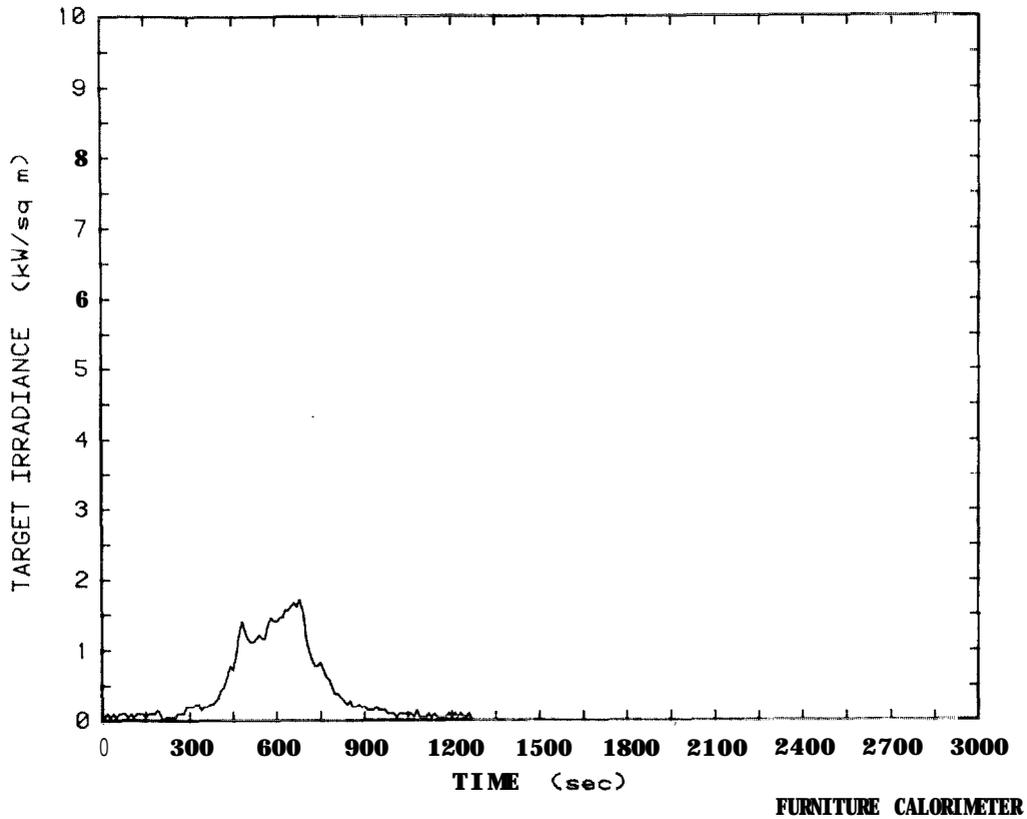
Figure 71. Target irradiance plot for metal. frame loveseat, Test 54
