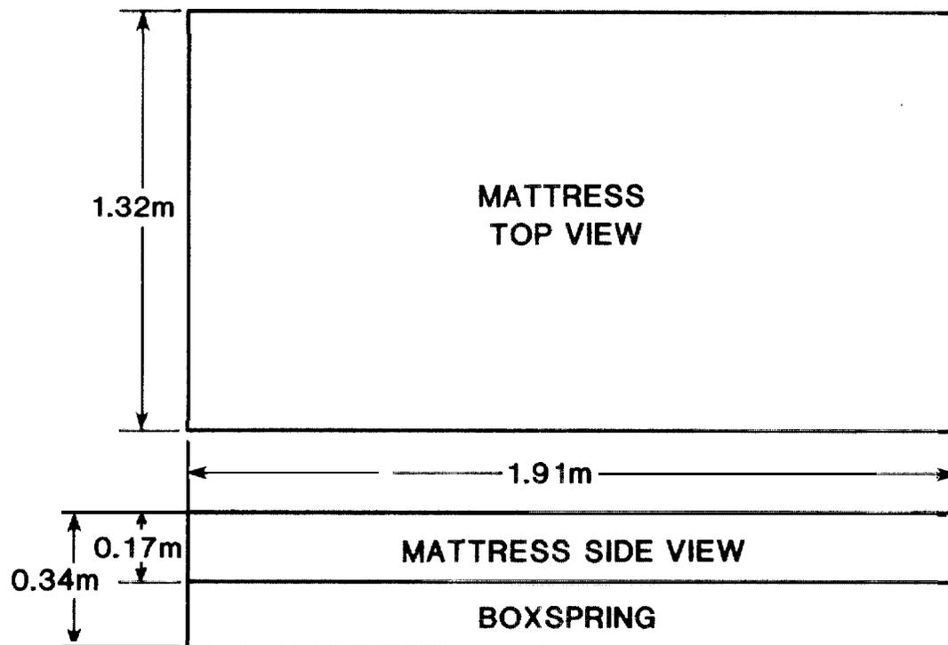
Figure 78. Photograph and dimensions of mattress and boxspring, test 67
